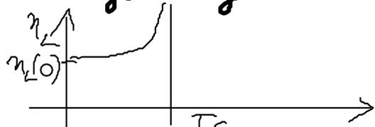
Bem.  $n_L(T) \sim \frac{1}{T n_s}$  Typisch  $n_L(0) \sim 100 \text{ \AA}$
