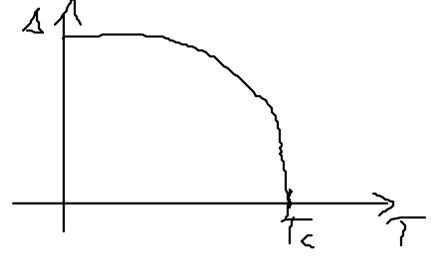
②  $k T_c = 1,13 \hbar \omega_c \exp\left[-\frac{1}{D(E_F) V_0}\right]$
