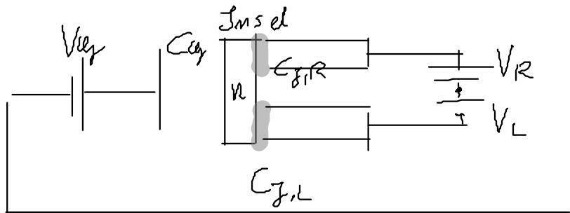
$$Q_g = C_g V_g + C_{jl} V_L + C_{jr} V_R$$
